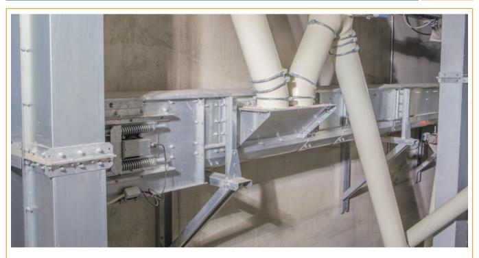
The purpose of the **PETKUS Round Bottom Chain Conveyor RF 250** is the homogenous transport of free flowing, bulky products such as grain, pulses, oilseeds and similar agricultural products.
