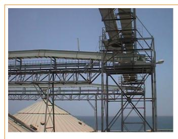
The purpose of the **PETKUS Trough Chain Conveyor TK 400 / TK 520** is the horizontal transport of free flowing, bulky products such as grain, pulses, oilseeds and similar agricultural products.
