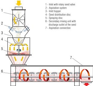
The **PETKUS Chemical Seed Treater CT 25** is used for continuous, wet Chemical Treating of seed such as grain, corn, pulses etc.
