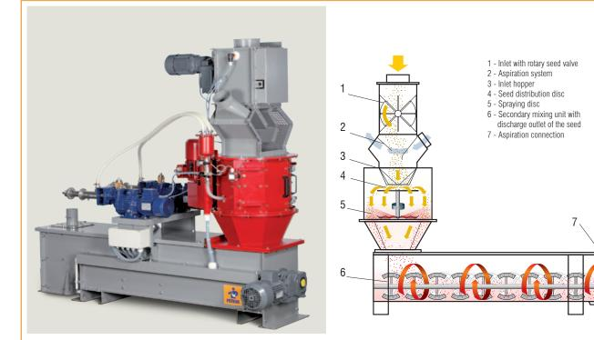
The **PETKUS Chemical Seed Treater CT 10** is used for continuous, wet chemical treating of seed such as grain, corn, pulses etc.
